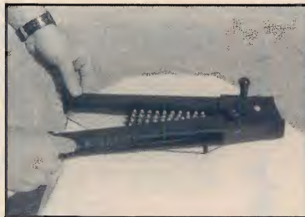
The M-900 magazine speed loader permits the loading of a magazine in as little as 30 seconds.
